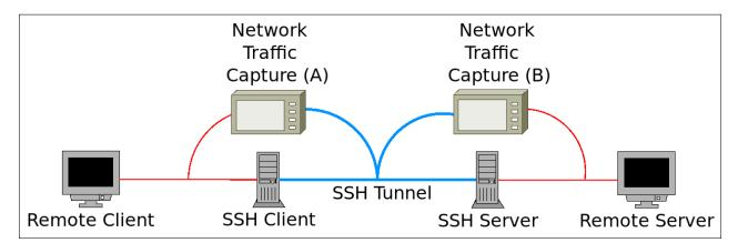
Figure 3.5: When analyzing a stream of SSH encrypted traffic for side-channels, the plaintext and corresponding encrypted stream may be captured at A or B.
