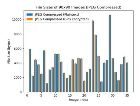
Figure 2.2: The size of the encrypted images closely follows the size of their plaintext counterparts.
