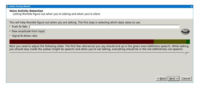
Figure 5.5: The Mumble client can be configured to only transmit when audio *amplitude* exceeds a *threshold* level.
