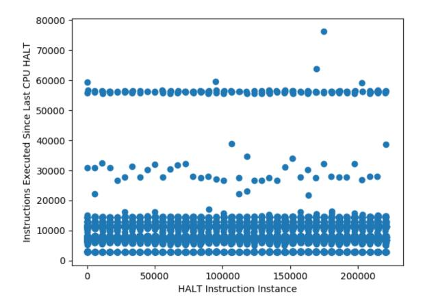
Figure 5.8: When the minimal Linux operating system is executing a CPU consuming userspace process, instruction segments of lengths that lie outside the *idle* cluster occur.
