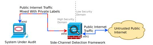
Figure 3.2: An example deployment of the framework for auditing network traffic for sidechannel information leaks. Network traffic is labelled with private activity. These labels are used for model training by the framework and then discarded.
