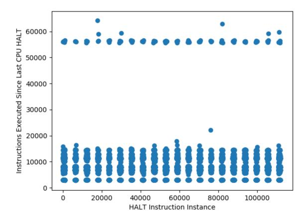
Figure 5.7: When the minimal Linux operating system is idle, lengths of sections of instructions processed between HALTs can be clustered in the regions of 0 to 20000 instructions and around 57500 instructions.
