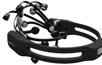
Figure 4.6: Emotiv Epoc headset used to collect EEG data in the Password Recall study [38].
