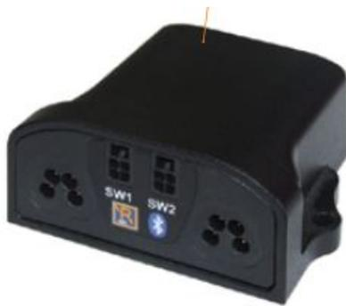
Figure 3.3: R-Net Encoder Module [5]
