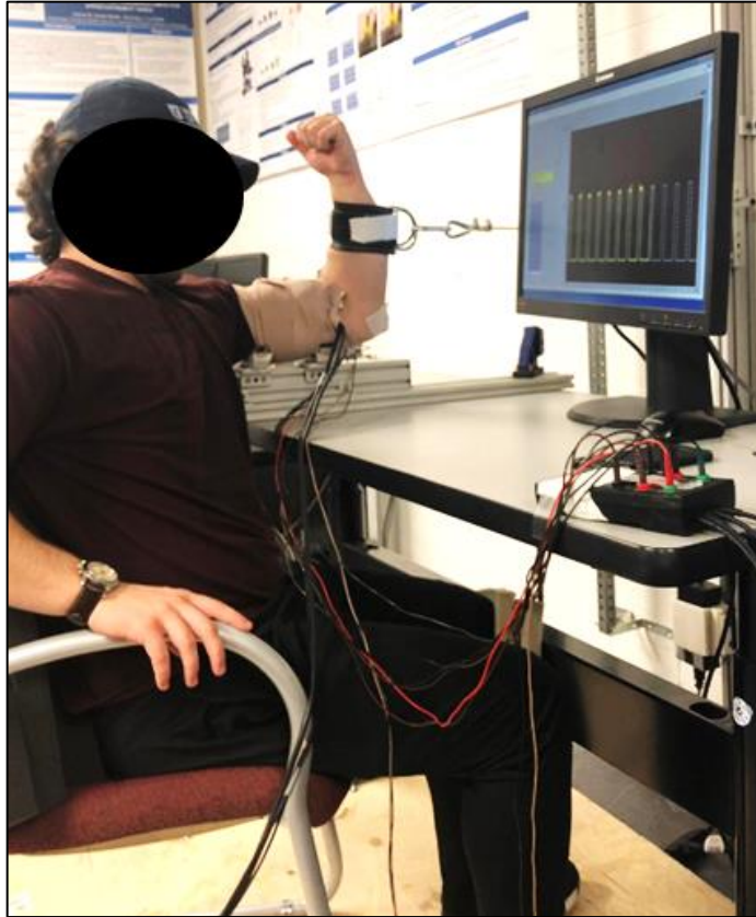
Figure 4.2: Experimental set-up. Participants were seated in front of a computer monitor, which provided online information on their force output relative to a template representative of the DC/TLV workload being conducted in that session.
