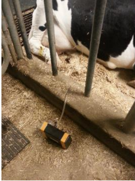
Figure 2.6. LeMotte Air pump is used with Tenax sorbent tube at 1.5 LPM for 5 minutes for VOC sample collection.
