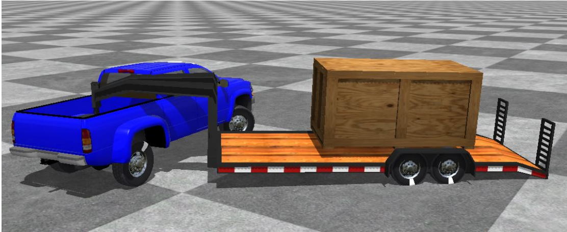
FIGURE 1.2: Pickup truck-trailer combination jackknife scenario
