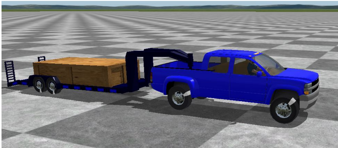
FIGURE 3.3: Configuration of a pickup truck with a tandem-axle gooseneck trailer in TruckSim
