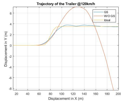
FIGURE 6.58: GSC Trajectory of the trailer at 120 km/h and 0.1(s) driver model reaction time.
