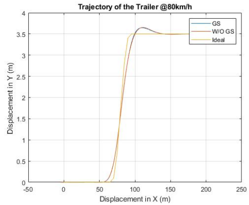
FIGURE 6.42: GSC Trajectory of the trailer at 80 km/h and 0.0(s) driver model reaction time.
