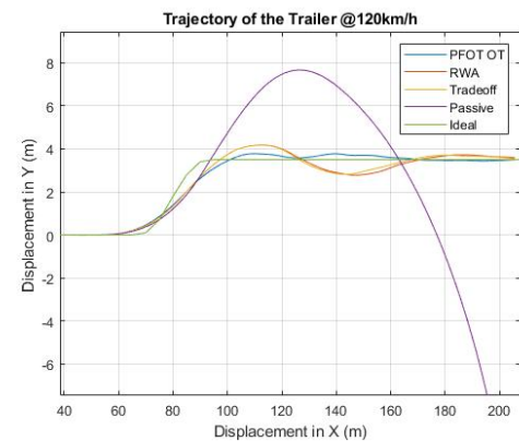
FIGURE 6.40: Trajectory of the trailer at 120 km/h and 0.1(s) driver model reaction time.
