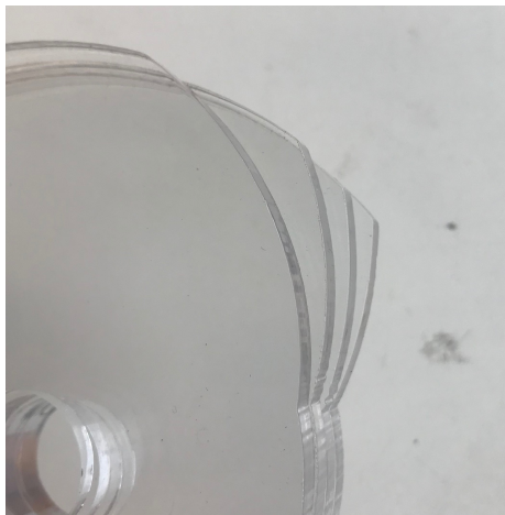
Figure 3.8: From top to bottom 20, 30, 35, and 40 degree constant pressure angle cam profiles
