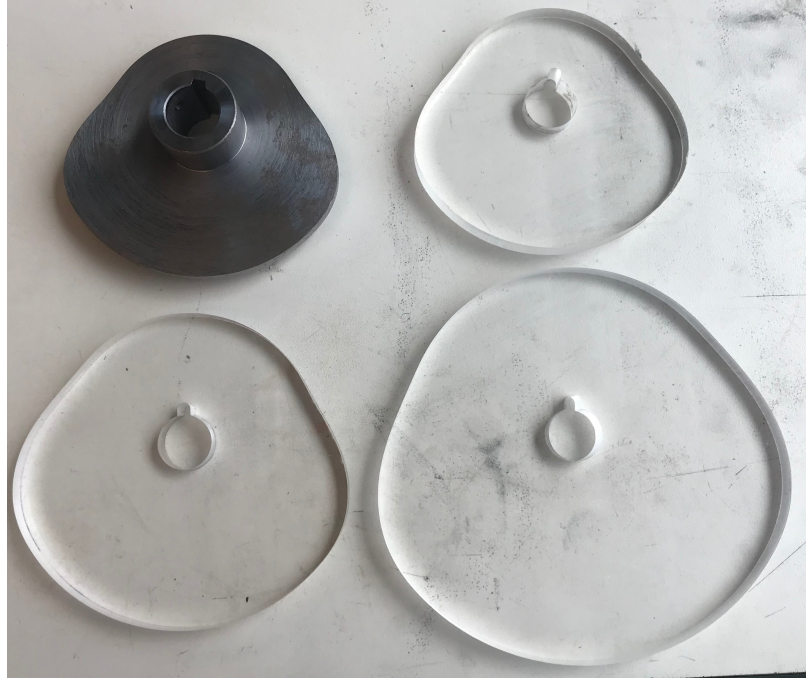
Figure 3.6: Polynomial steel and acrylic cam profiles: 30, 30, 25, and 20 degrees from top left to bottom right)
