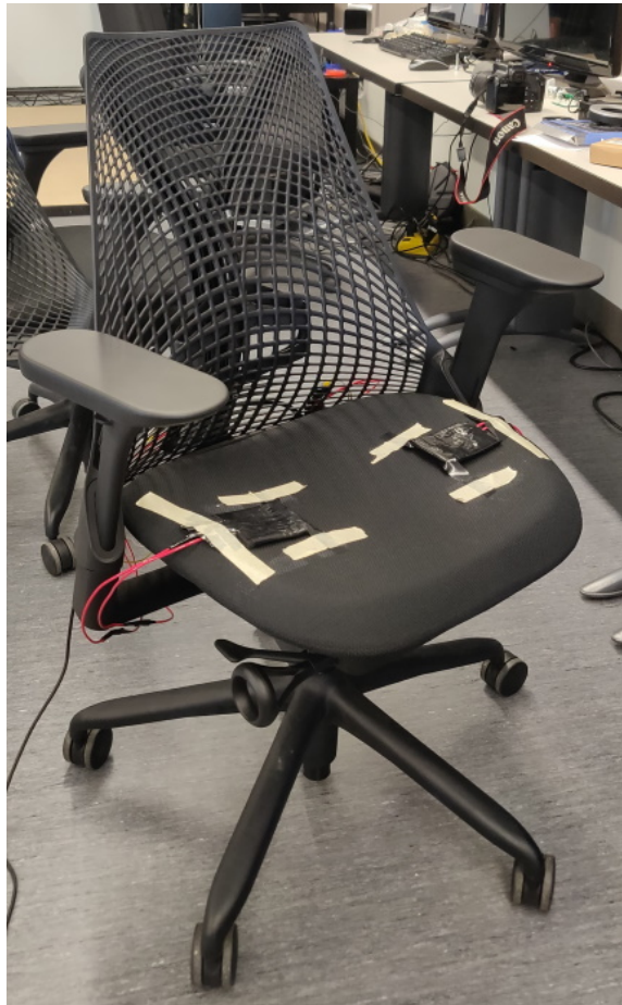
Figure 3.3: Full SeatController prototype with custom made pressure sensors affixed to the seat.
