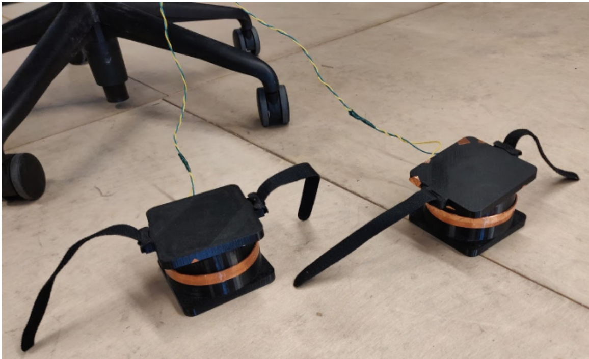
Figure 3.9: The Spring Stepper device when assembled and connected to the Arduino Uno, which is mounted on the back of the swivel chair.
