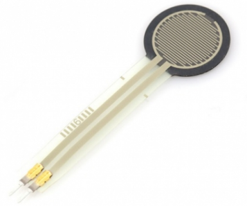
Figure 3.6: Force-sensitive resistor used with the Home Hiker prototype.
