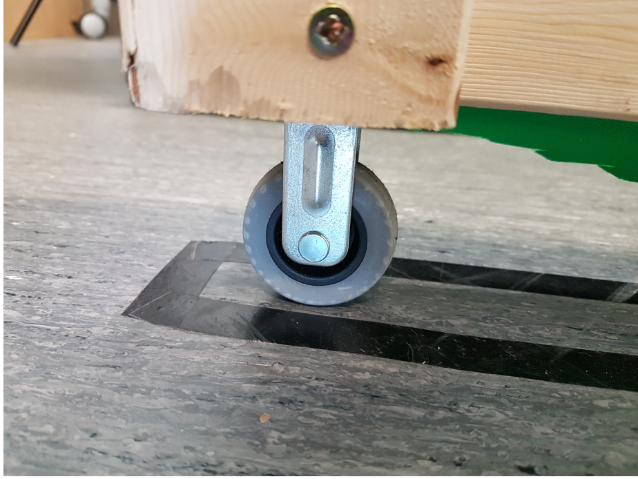
Figure 4.3: Rigid casters allow the green screen chamber to move forward and backward linearly, for accessing the driving simulator.
