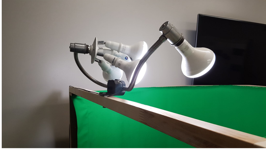
Figure 4.2: Flood lights mounted to the green screen chamber. They are angled to light all sides of the chamber.
