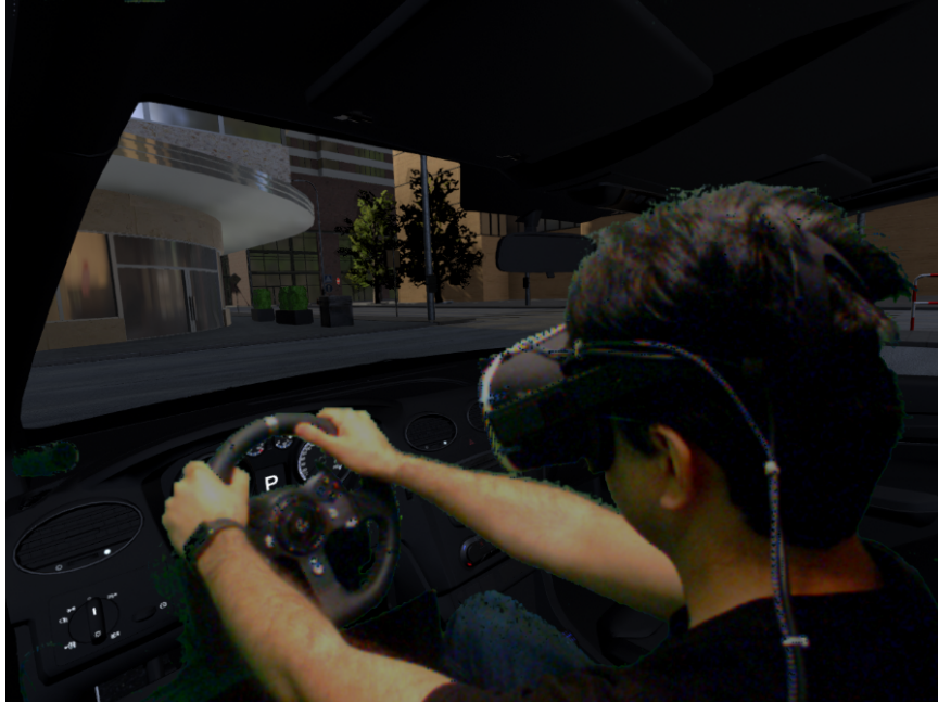
Figure 3.7: A third-person view of a user driving the simulator in front of a green screen, composited with the virtual vehicle.
