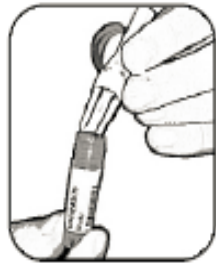
Step 2: Place ribbed-end of the SCA securely into a pre-labeled collection vial (see Caution 3 above).
