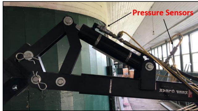
Figure 3-12: Pressure sensor location
