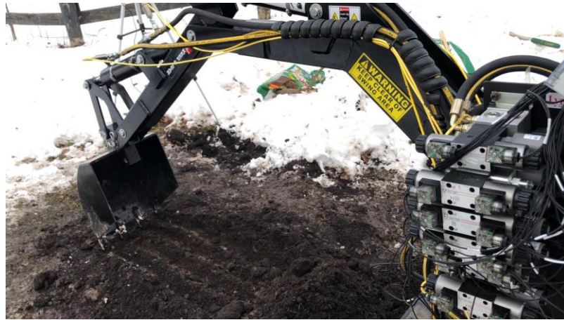
Figure 7-2: Ground levelling experiment with prototype excavator
