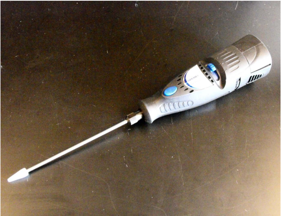
A Dremel® 4.8V MiniMite Cordless with a custom conical blending attachment, used to homogenize ferments.
