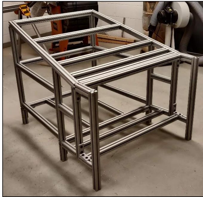
Figure 3.5 Internal structure to support testbench
