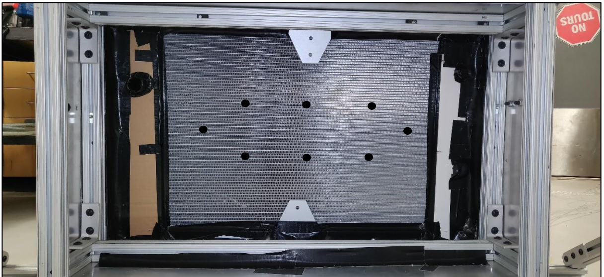
Figure 3.11 Radiator installed in testbench and sealed
