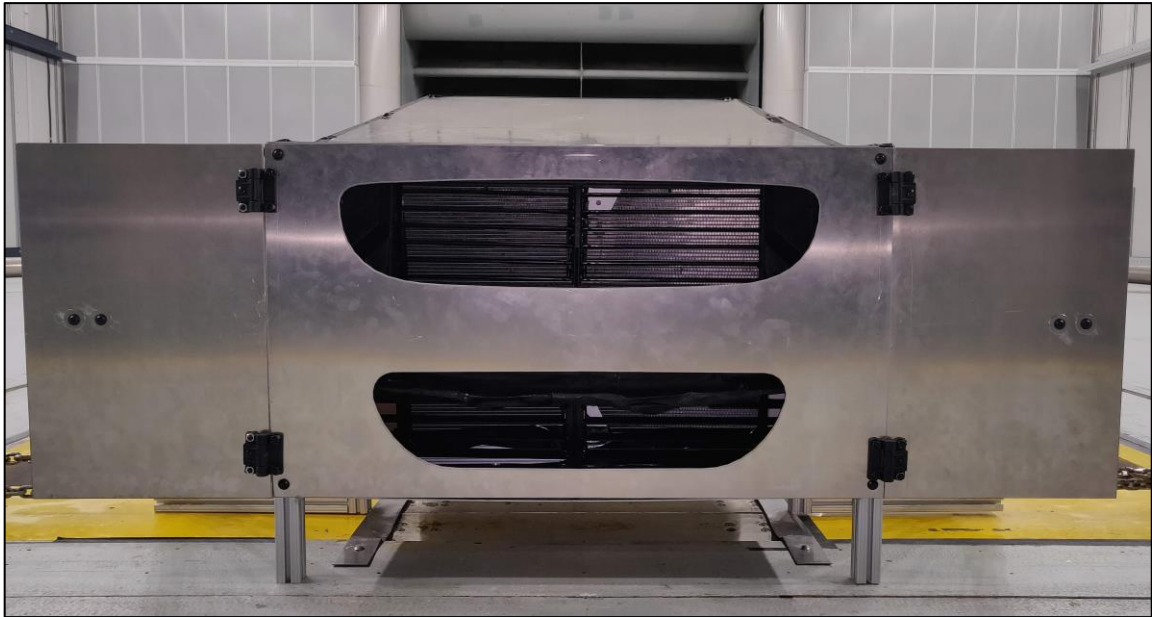
Figure 4.2 AGS fully open
