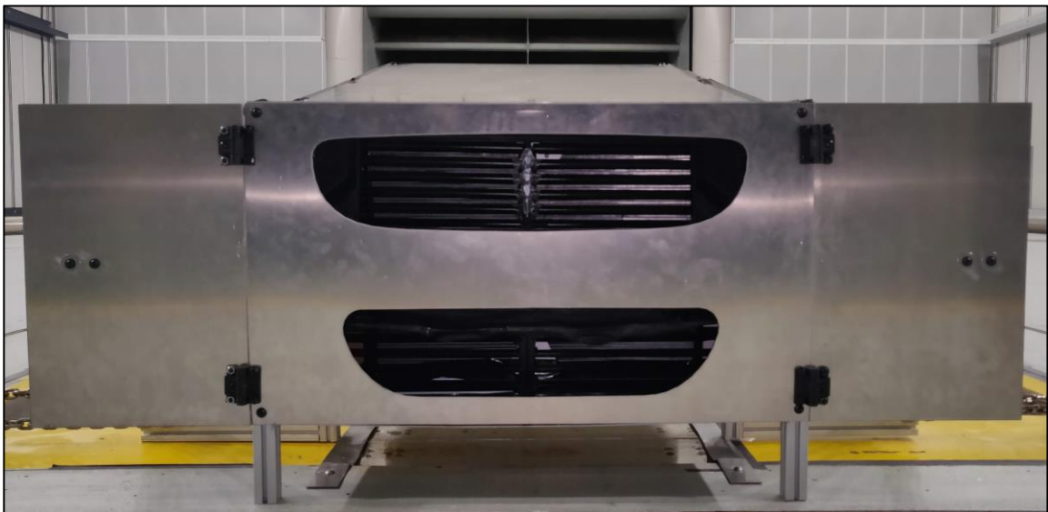
Figure 4.3 AGS partially open
