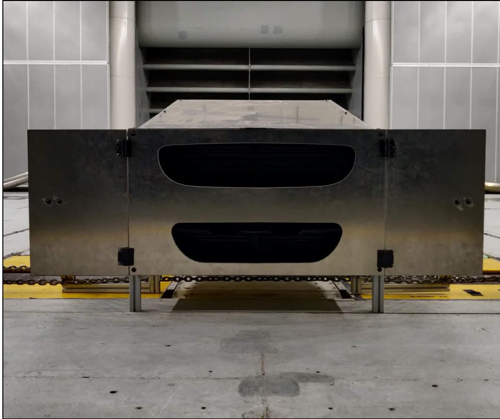
Figure 3.13 Front fascia installed on testbench
