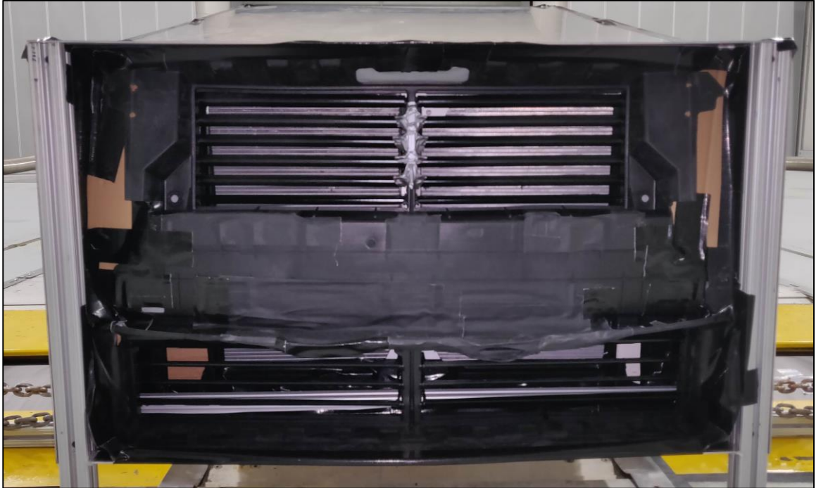
Figure 3.12 AGS installed in testbench and sealed
