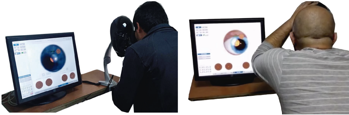
Figure 3: The EYESi DO simulator in use. The monitor shows what the trainee is seeing while capturing performance metrics associated with the examination for assessment.
