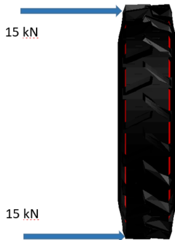
Figure 6-9: HLFS translational stiffness test with two 15 kN translational loads.
