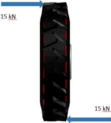
Figure 6-11: Rotational stiffness test using 15 kN lateral load.
