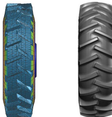
Figure 3-2: The HLFS agricultural tire made by Barez Tires [70] and its model in Pam-Crash.
