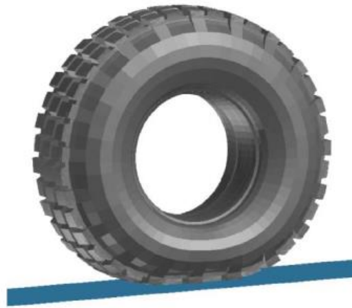
Figure 2-15: Hossam Ragheb's combat vehicle FEA tire model for an 8x8 combat vehicle [34].
