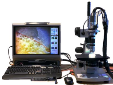
Figure 3.7: Digital Microscope – DM (VHX – 1000).
