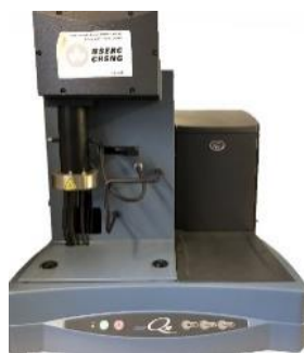
Figure 3.3: Thermo-gravimetric Analyzer - TGA (Q series – Q50).
