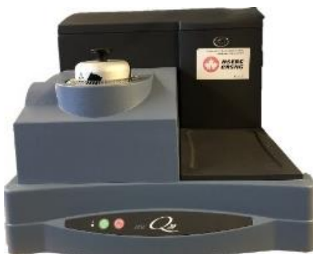
Figure 3.4: Differential Scanning Calorimeter - DSC (Q series – Q20).
