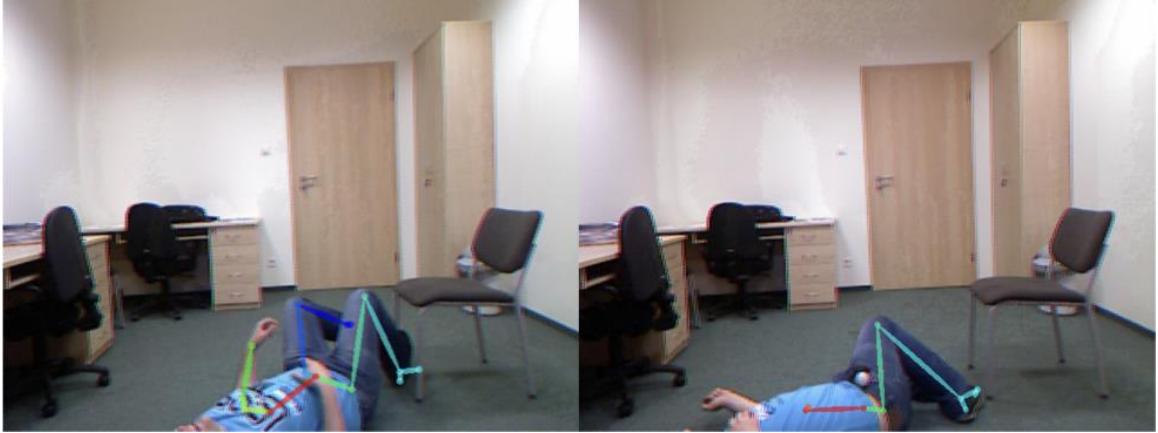
Figure 6.4: OpenPose misses detecting body keypoints when occlusion happens. [21]
