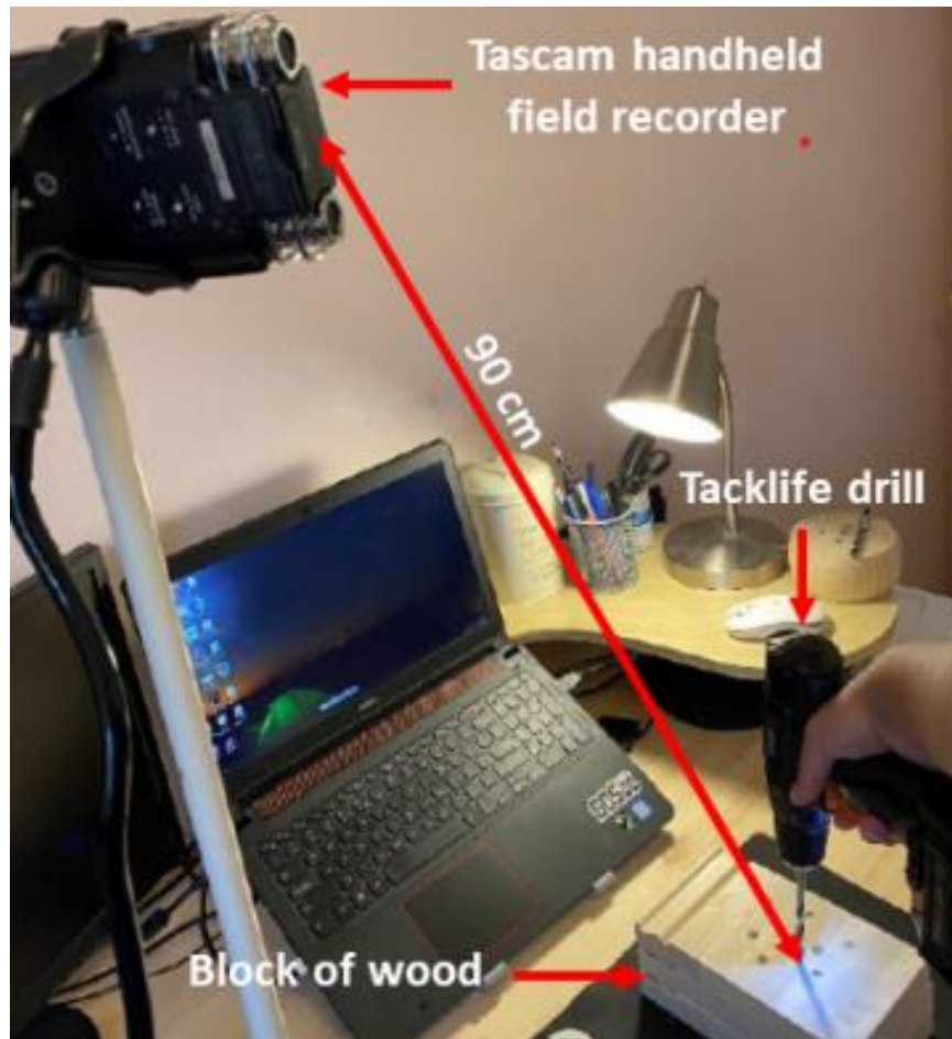
Figure 3.1: Auditory stimuli recording setup.
