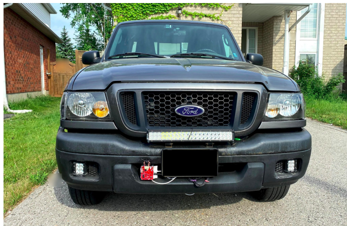
Figure 4.1: Radar and camera sensor placement on test vehicle
