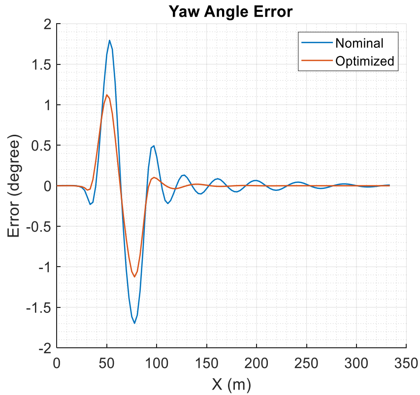
Figure 4.6: Yaw angle deviation in highway scenario.
