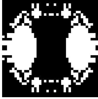
Figure 3.48 – Results of minimizing ratio of first natural frequency to the average of six first natural frequencies and constraint on a minimum of first natural frequency.
