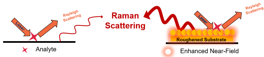
Figure 1.5. Schematic diagram of the established SERS method
