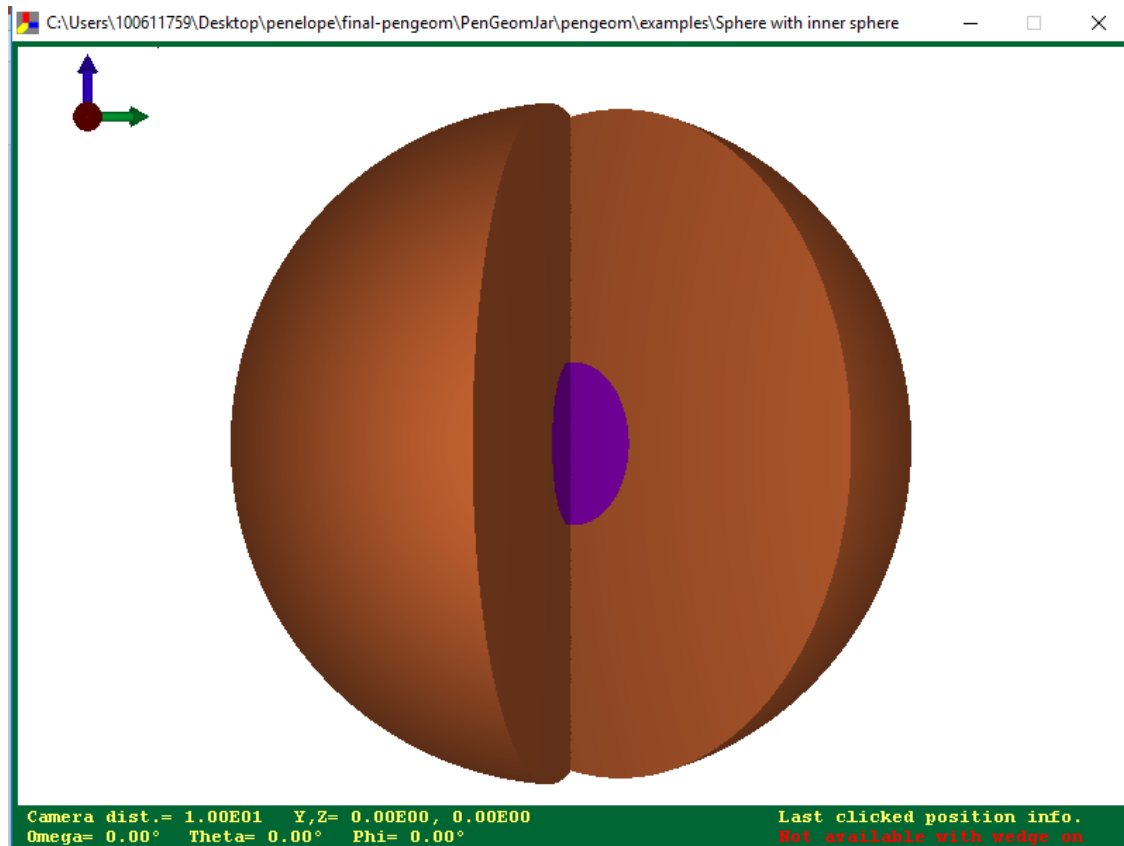
FIGURE 3.7: 3D view simulating the experimental set up used by Kliauga and Dvorak (1978), MAT1: 2.54cm diameter grid wall-less counter, surrounded by MAT2: a 10.2cm spherical shell. The wedged out portion exposes MAT2 [18]
