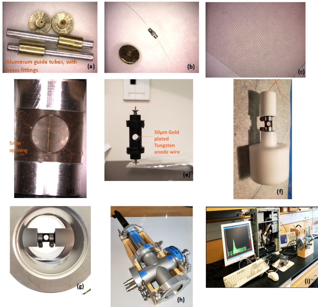
FIGURE 4.8: A montage of the assembly parts for use in the design and construction of a cylindrical type Wall-less TEPC: (a) Magnified image of 2 mm diameter anode potential guide tubes, with brass fittings; (b) magnified image 50 \mu\text{m} gold plated tungsten anode wire; (c) 30 mm x 30 mm copper mesh with 88% transparency; (d) mesh attached to the body of the A150 plastic column to form the cathode, with a 5 mm opening; (e) partial assembly of the counter;(f) counter affixed to holder for insertion into the vacuum chamber;(g) partial assembly in vacuum chamber;(h) full assembly of chamber with detector positioned in side, and perpendicular to the plunger holding the source; (i)current architecture for collecting results.
