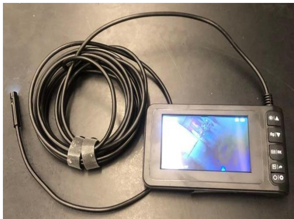
Figure 3.8: YINAMA Dual-Lens Digital Borescope.
