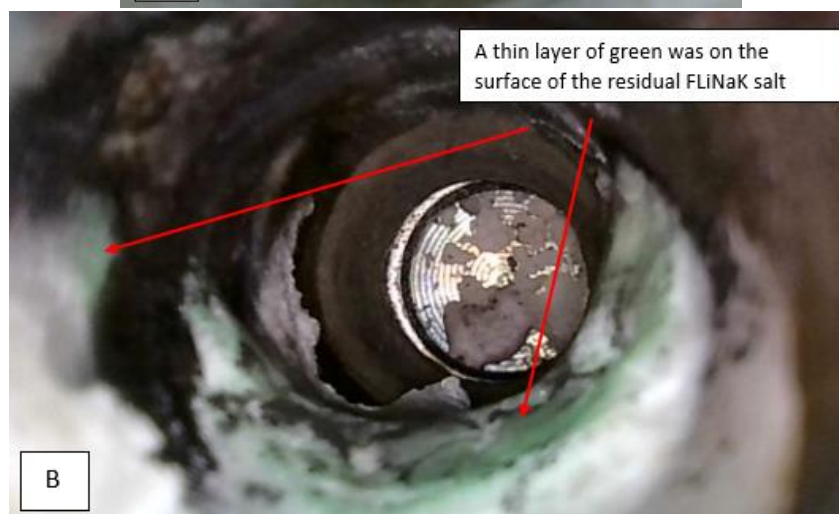
Figure 4.69 (a): Large, Thick Patches of FLiNaK was Observed on One Side of the Tube Wall (b): A Thin Layer of Green Hues was Observed on the Surface of the Salt.
