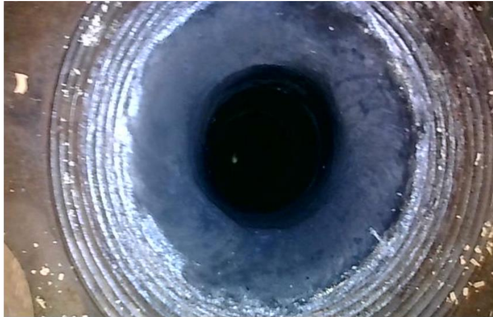
The Hastelloy at the top opening of the MSL Tube Segment had become blackened and dull
