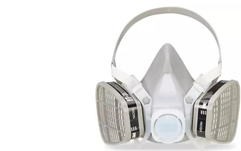
Figure A.3: N100 Respirator used for experiments involving any handling of FLiNaK
