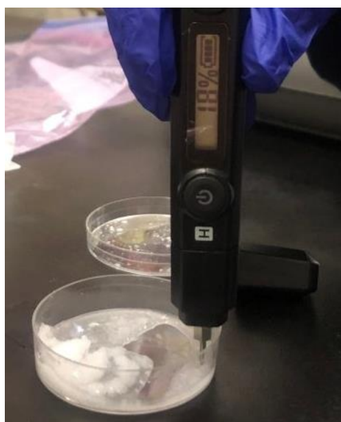
Figure 2.31: The conductivity of the aqueous solution formed as a result of FLiNaK deliquescence in % IACS
