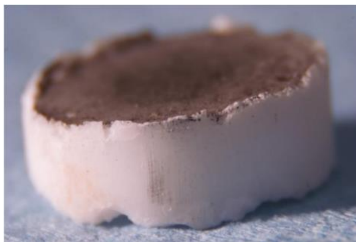
Figure 2.29: Initial Conditions of Furnace Synthesized FLiNaK Sample.
