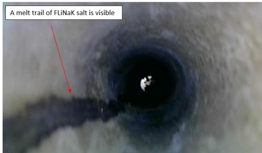
Figure 4.68: Photo of Zone 4 with Salt Plug Melting Trail.
