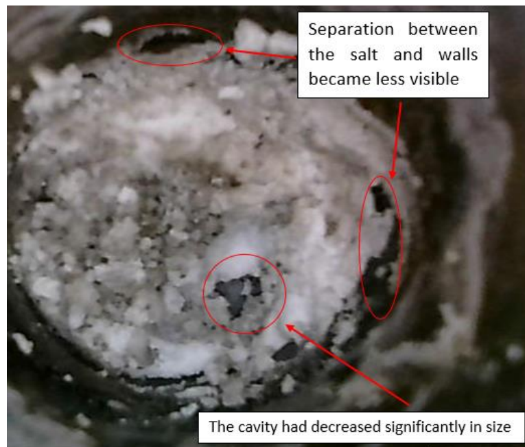
Figure 4.58: There was a small cavity left on Side-A and the salt appeared dark grey.
