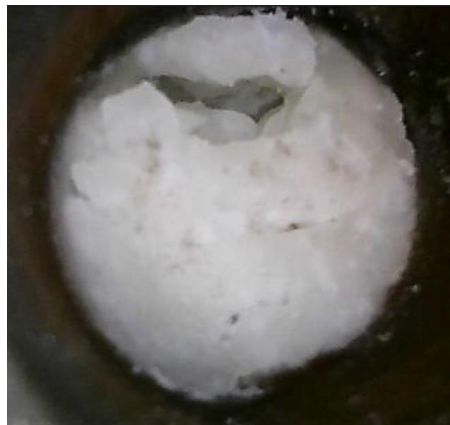
Figure 4.52: Borescope Photo of Side-A of the Salt Plug - Second Trial.
