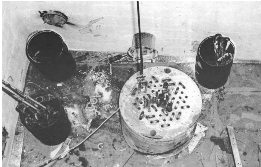
Figure 2.6: Top of the Reactor with the Pressure Shell and Some Fuel Tubes Removed [30].
