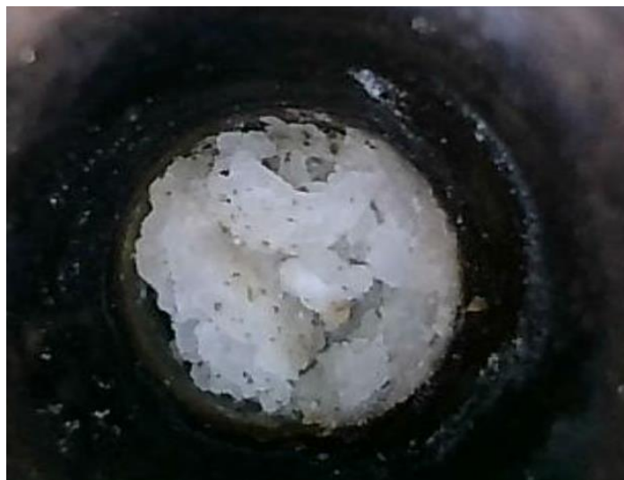
Figure 4.53: Borescope Photo of Side-B of the Salt Plug - Second Trial.
