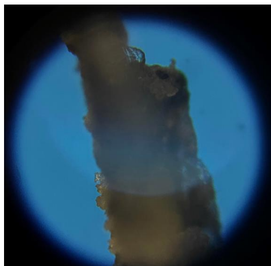
Figure 4.73: Photo of Twisted Strip under 40X Magnification- the Midsection was Dull.
