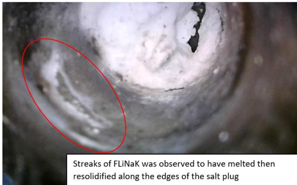
Figure 4.49: The Salt Plug Had Melted along the Walls of the Tube Segment.
