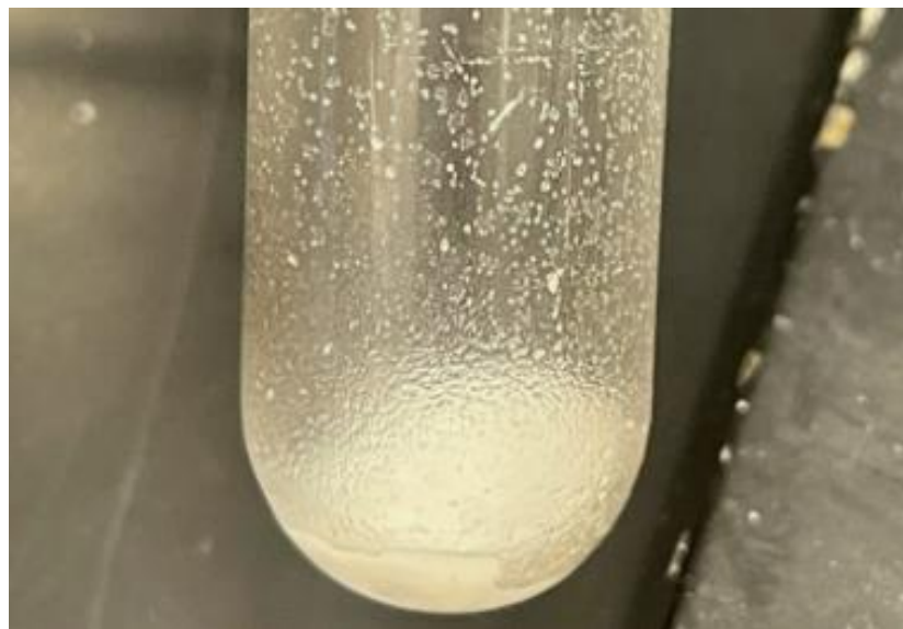
Figure 4.26: Photos of Sample B-3 from Different Angles - the measuring tape sticker was temporarily removed to better capture the presence of water and salt migration.
