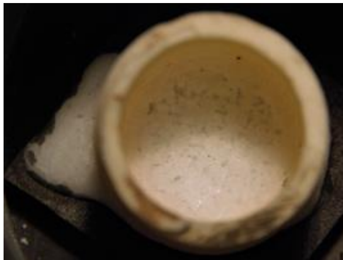
Figure 2.28: Synthesized FLiNaK in Ceramic and Graphite Container.
