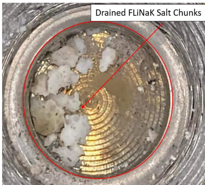
Figure 4.61: Close-up Photo of the Drained Salt Chunks.
