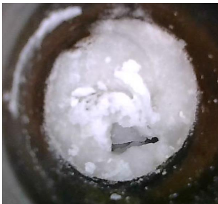
Figure 4.44: Increased Moisture in the Summer Caused the Surface of Side-A to Become Smooth and Translucent.
