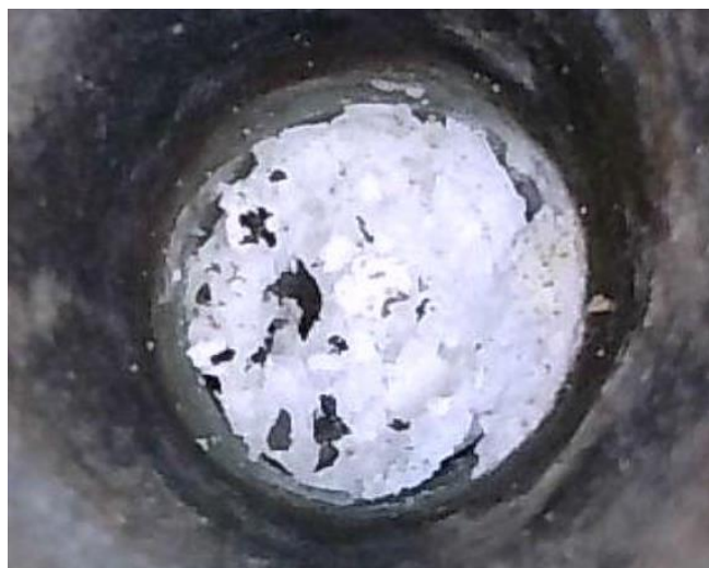
Figure 4.59: Very Large Flakes of Black Contaminant were Found Amongst the Crystals.
