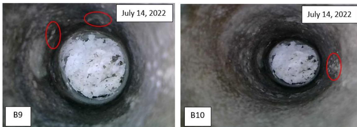
Figure 4.71: Progression in Salt Migration Severity on Side-B of the Salt Plug from May 2021 to July 2022.
