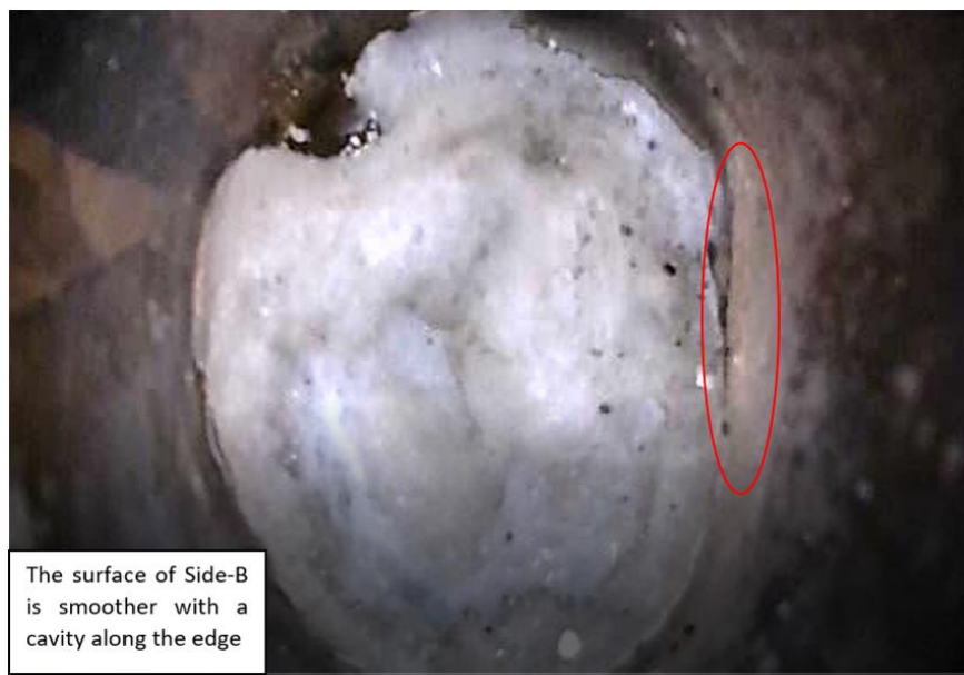
Figure 4.42: Side-B of the Salt Plug Features a Small Cavity Along the Hastelloy Wall.
