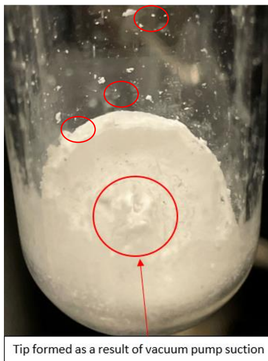
Figure 4.13: Sample A-3 Showing Signs of Salt Migration as Salt Crystals begin Detaching and Reattaching Away from the Main Salt Mass.
