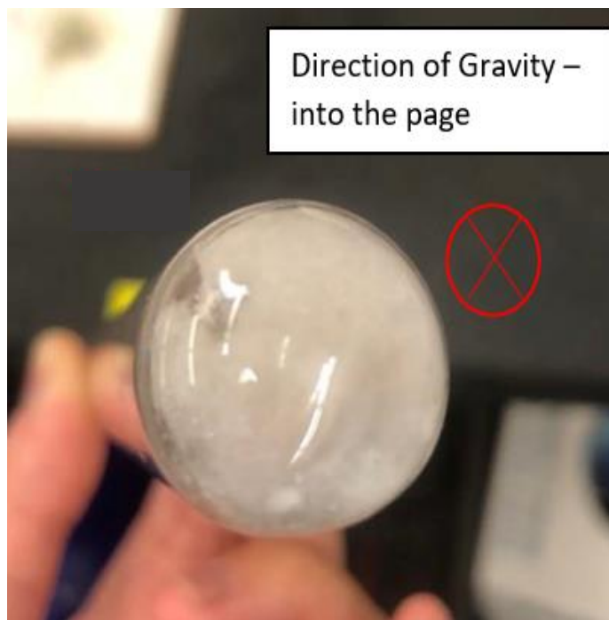
Figure 4.7: The FLiNaK sample had stuck to the bottom and walls of the test tube and could not be removed.
