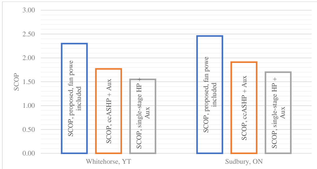
Figure 4.18: SCOP comparison for systems running in Whitehorse, YT and Sudbury, ON: 1) proposed system, fan power included, 2) ccASHP unit plus auxiliary electric heating, and 3) Energy Star single-stage system plus auxiliary electric heating.
