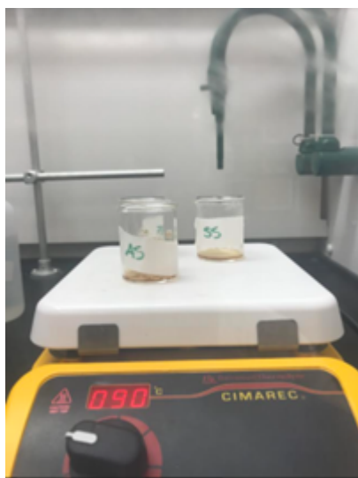
FIGURE 3.5: Samples undergoing the open-vessel digestion process on a hot plate in the fume hood.
