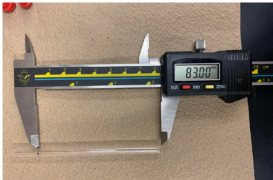
FIGURE 3.10: Using digital calipers to mark EPR tubes at heights of 8.3 cm and 3.4 cm.
