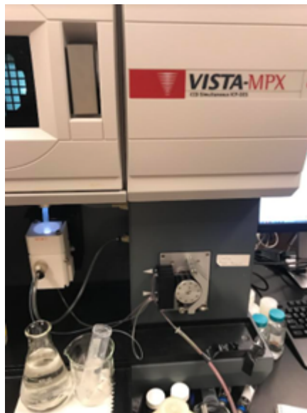
FIGURE 3.9: Sample being analyzed with the Vista-MPX ICP-OES.
