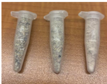
FIGURE 3.4: Shell powder of various sizes (From L-R: 1-0.5mm grain size, 0.5-0.1mm grain size, >0.1mm grain size).
