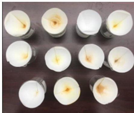
FIGURE 3.8: Dried filter papers with leftover shell residue to be weighed.
