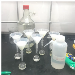
FIGURE 3.6: Samples filtering into volumetric flasks through filter paper.
