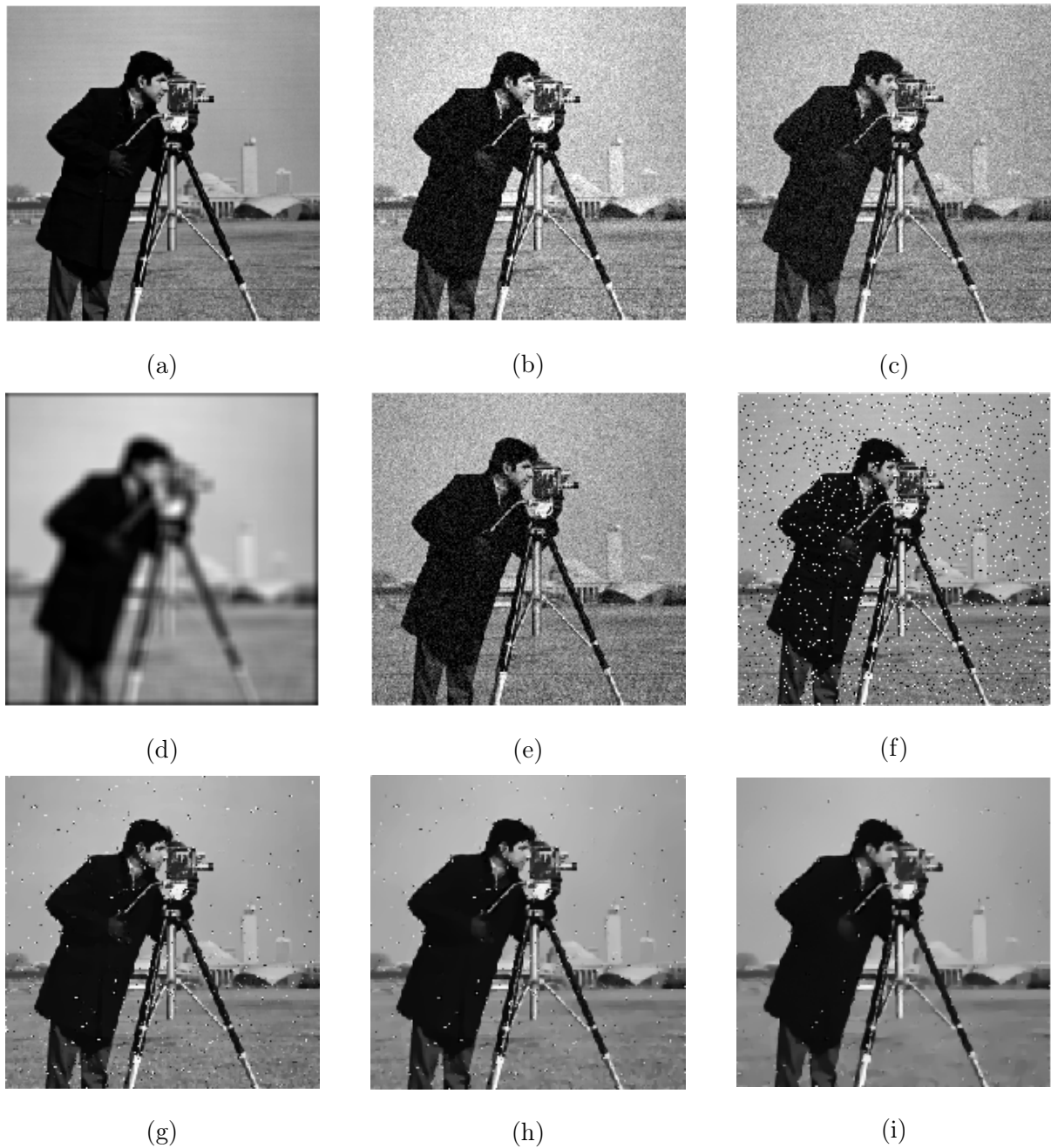
Figure 5.23: Visual results for the fusion of a set of distortion versions of the test image Cameraman. (a) Original image. (b) Gaussian noisy mean contrast Stretched. (c) Gaussian noisy mean shifted. (d) Blurring. (e) Gaussian noise. (f) Salt and pepper noise. (g) Fused image ( \lambda = 3.5 ). (h) Fused image ( \lambda = 7 ). (i) Fused image ( \lambda = 14 ). (The starting point is the salt and pepper noisy image).
