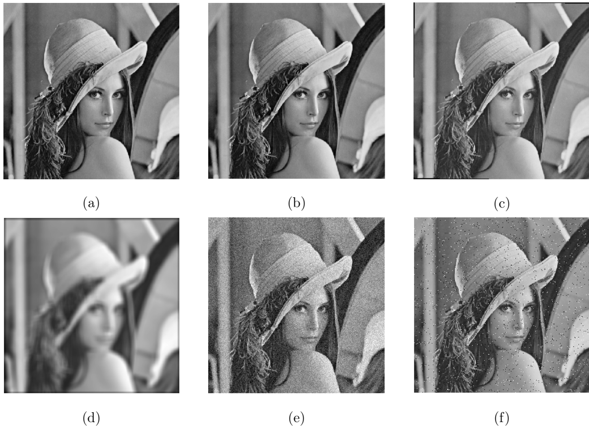
Figure 2.2: Comparison of distorted images with the same MSE. (a) Original image (MSE=0;SSIM=1); (b) Shift (to the left) (MSE=400;SSIM=0.97); (c) Rotation (clock-wise) (MSE=430.24;SSIM=0.67); (d) Blurring (MSE=402;SSIM=0.62); (e) Gaussian noise (MSE=400;SSIM=0.34); (f) Salt and pepper noise (MSE=402;SSIM=0.57);
