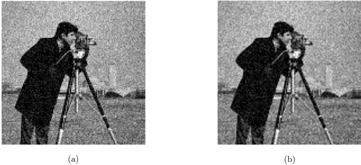
Figure 5.28: Visual results of one of the noisy images and resized version of it. a) The Cameraman's image is degraded by local averaging followed by a downsampling factor of two and Gaussian noise. (b) The resized version of the distorted image (a) by applying bicubic interpolation.
