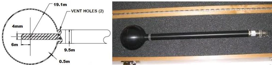
Figure 4-2 Standard Imaging A4-ionization chamber, collecting volume: 30cc
