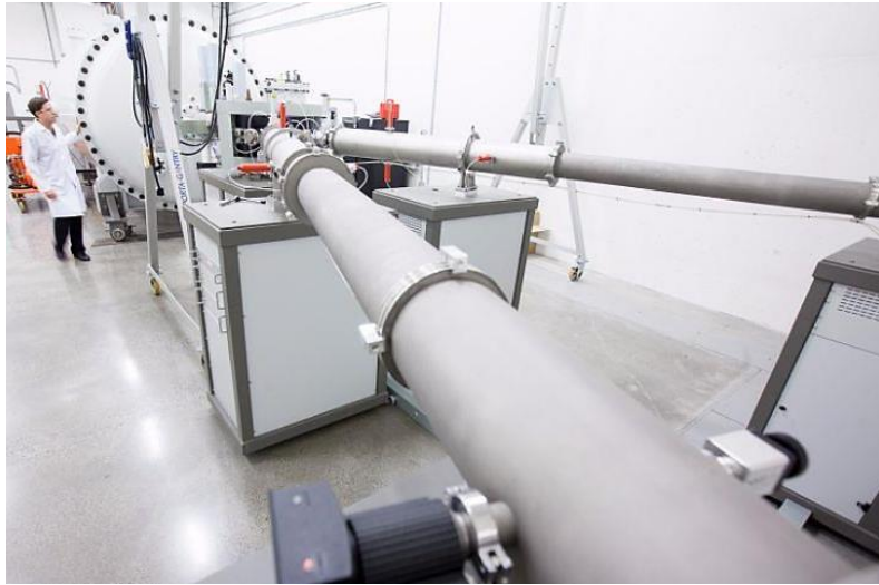
Figure 8-2 Beam lines directing the charged particles beams to the target rooms (RMTL, 2015).
