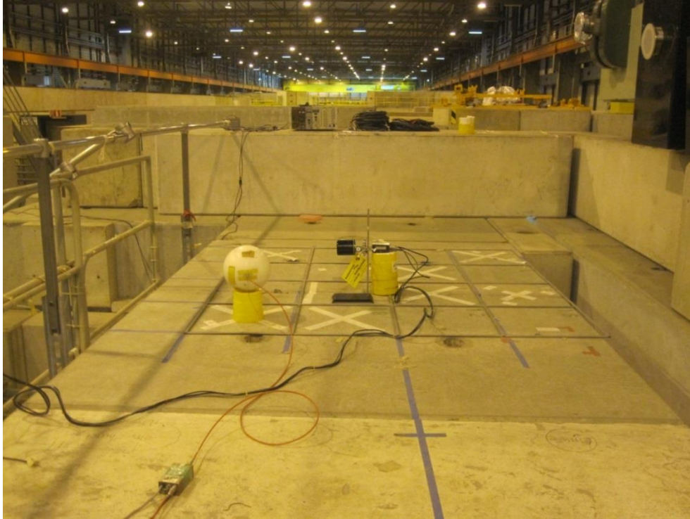
Figure 9-2 Iron shield roof above the target, gridded for radiation measurements at CERF.
