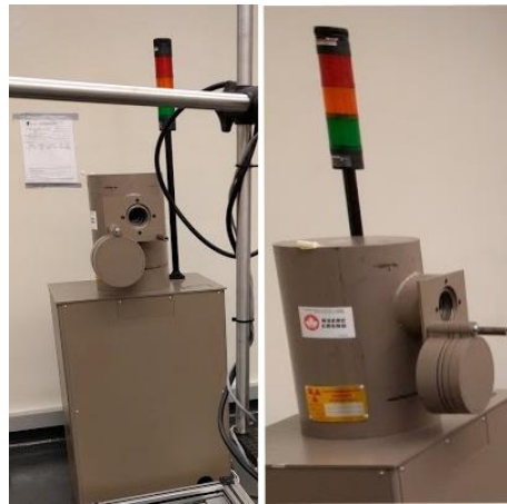
Figure 4-10 G10 - gamma Irradiator with a source of Cs-137
