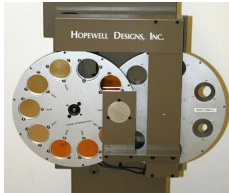
Figure 4-9 X80 - X-Ray Beam Irradiator, the filter wheels and the shutter
