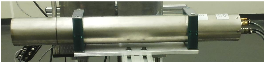
Figure 4-11 P385 - Neutron Generator (Thermo-Fisher Scientific)
