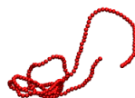
FIGURE 4.13: Pictures from simulation of a polymer getting stuck at the pore and getting bunched up. In this state, either end of the polymer could find the pore and thread through.
