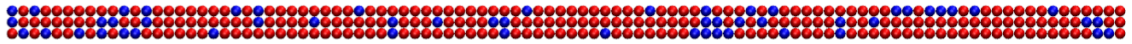
FIGURE 4.1: Picture of a possible configuration of singular defects. The beads coloured blue are defects. We set 20 % of the beads on the 3HB to be defective.
