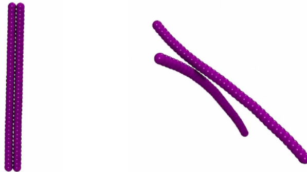
FIGURE 2.8: On the left are two rods we consider bundled. They are close enough together, and they are parallel. On the right are two rods which are close enough together, but do not satisfy the angle condition, and so we do not consider them bundled together.
