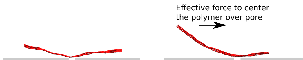
FIGURE 4.5: Closest Monomer to the pore over time, without a defect. Voltage significantly decreases the side to side motion.
