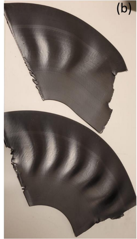
Figure 5.3: Flow imbalance during the sheet extrusion (a) sheet exiting from the die (b) collected sheet samples.
