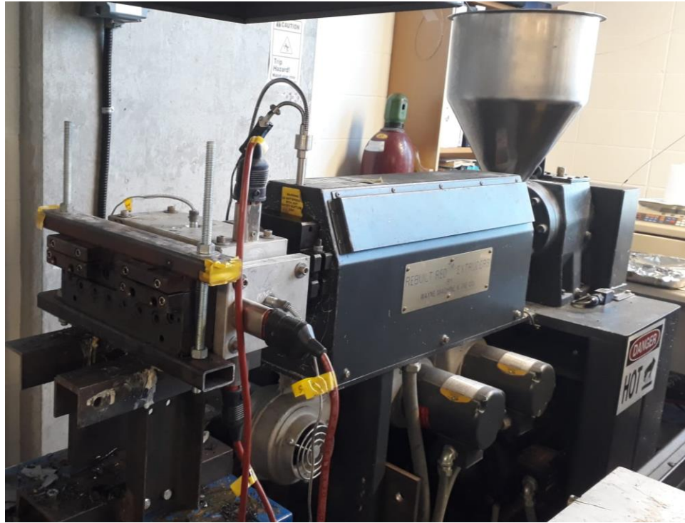
Figure 5.1: Single screw extruder for the sheet extrusion process.
