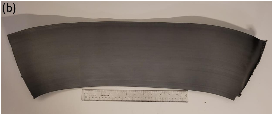
Figure 5.4: Sheet of the electrically conductive thermoplastic composites (a) coming out from sheet die (b) collected sample.
