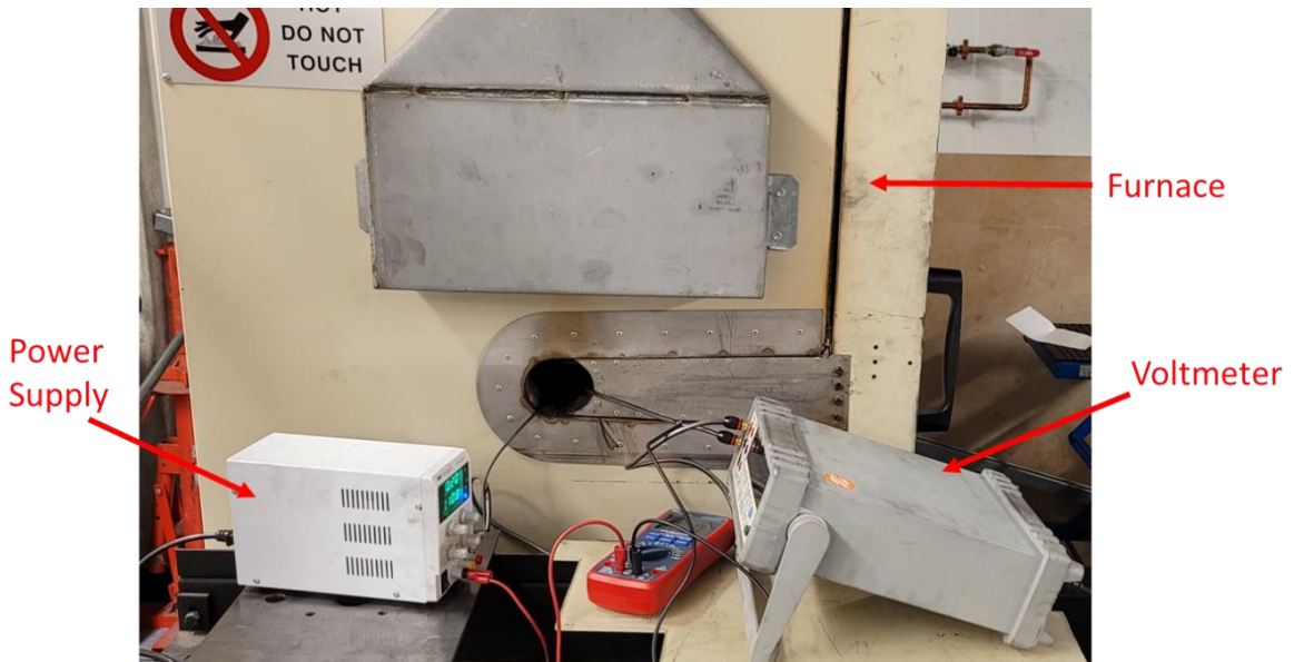
Figure 4.59: Electrical conductivity testing at variable temperature.
