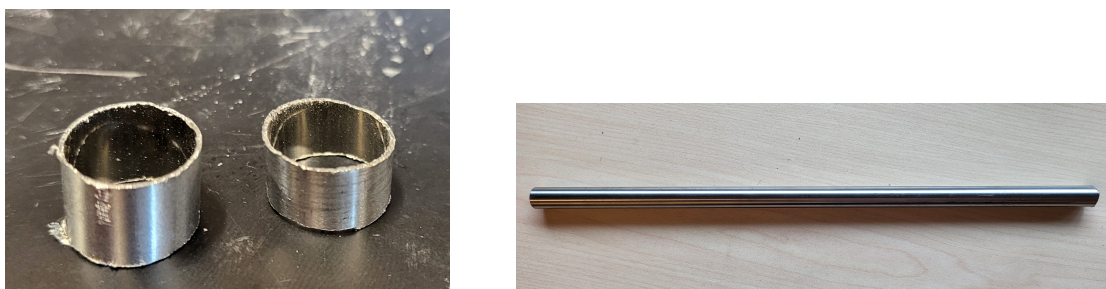
FIGURE 3.2: Images of the Zircaloy-4 samples used in the solubility experiments and the source cladding tube.
