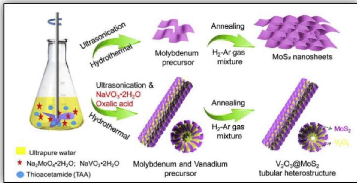
Figure 2-11: The schematic detailed diagram for the fabrication process of the \text{MoS}_2 nanosheets and the tubular (hollow) \text{V}_2\text{O}_3@/\text{MoS}_2 composites. Reprinted with permission from [133].
