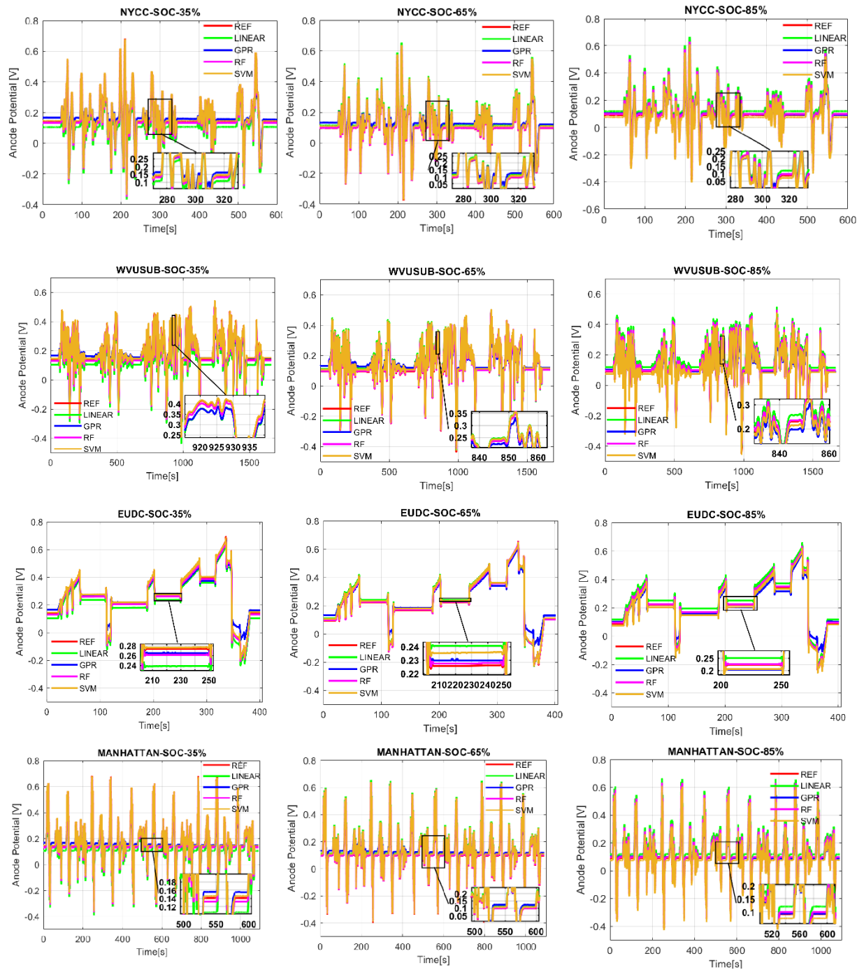
Figure 5-5: Anode Potential Predictions on the Test Data with the Initial SOC's of 35%, 65%, and 85% Using 4 Common Regression Algorithms. REF (red curve-Physics-based model), Linear regression (green curve), Gaussian process regression (blue curve), Random forests (pink curve), and Support vector regression (yellow curve).
