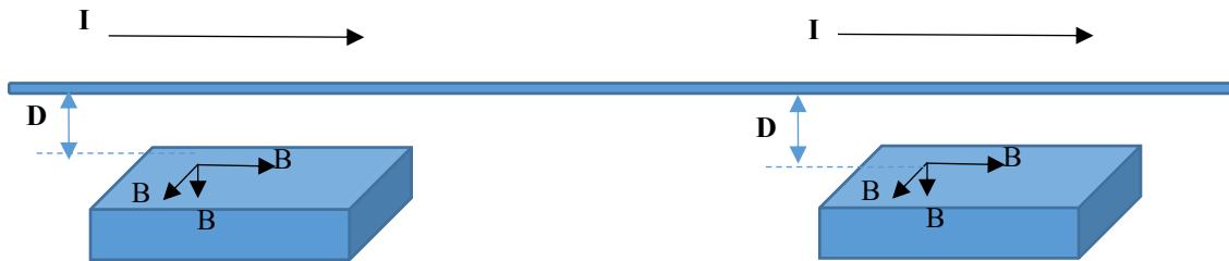
Figure B.8 Use of two sensors with measuring field, B_x in the direction of current flow
