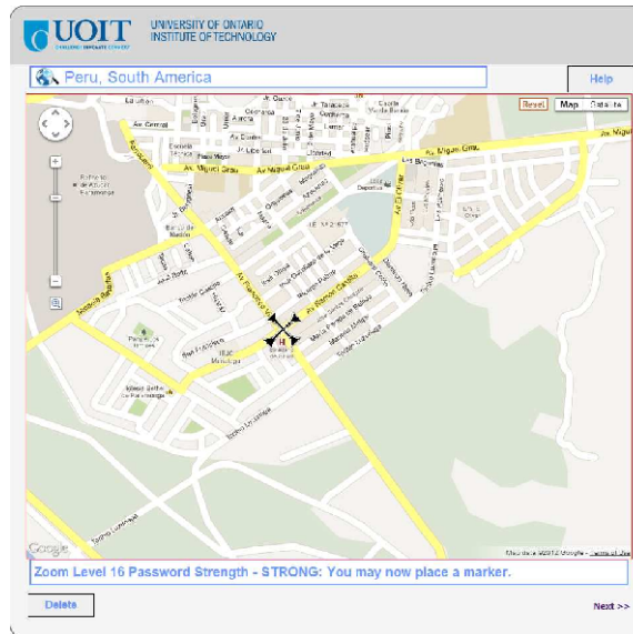
Figure 2.4: The user interface of GeoPass. Users need to select a location on a map as their passwords.
