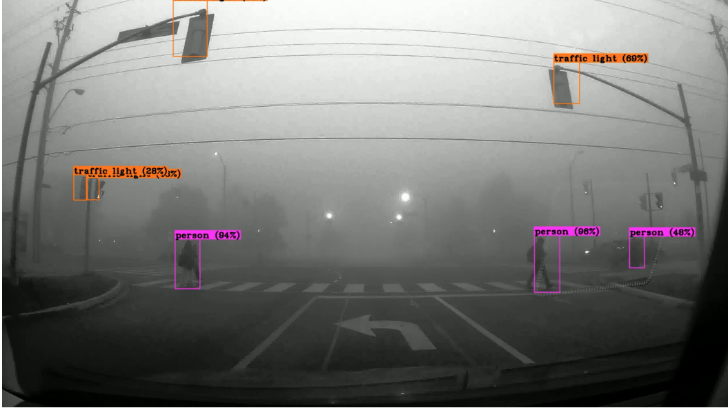
Figure 2.3: Using AHE method and YOLOv4
