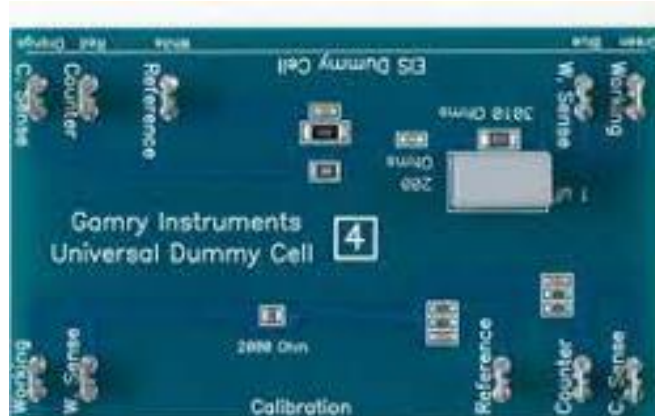
Figure 3.11 Gamry calibration configuration and Universal Dummy Cell [76]
