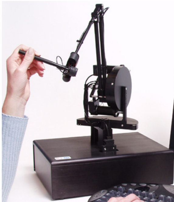
Figure 2.2: A Phantom Haptic Device offered by 3D Systems Inc., formerly SensAble. Image by 3DSystems
