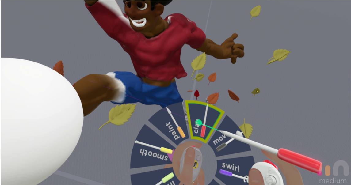
Figure 1.8: ‘Sculpting’ in Adobe Medium primarily involves applying 3D Boolean Operation CSG stamps to add or remove material. Note that the ‘tool’ in VR used to sculpt, which is attached directly to the hand. This ‘clay’ tool will continuously generate geometry at the tip of the pencil with a chosen stencil shape.
