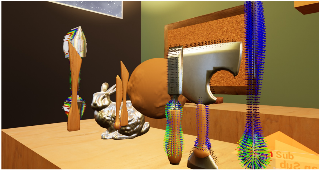
Figure 3.4: Vector fields visualized in different tools. Each vector field is constructed from the gradient of its SDF, and points outward toward the outside of the tool's surface. These vector fields are used in combination with the to linear and torque forces to determine how the tool will push clay. This model is independent of the geometry of the tool, allowing any shape of 3D object to be converted into a tool.
