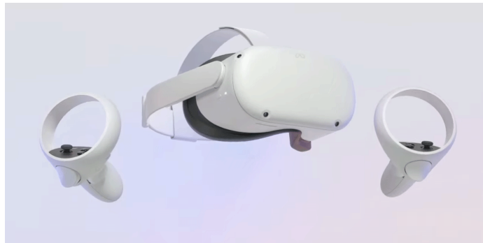
Figure 2.5: A Meta Quest 2 VR system with controllers, image by Meta Platforms Inc. This particular system uses inside-out tracking, processing depth information of the surrounding stationary environment relative to several cameras on the headset to determine the headset and controllers' position and orientation.
