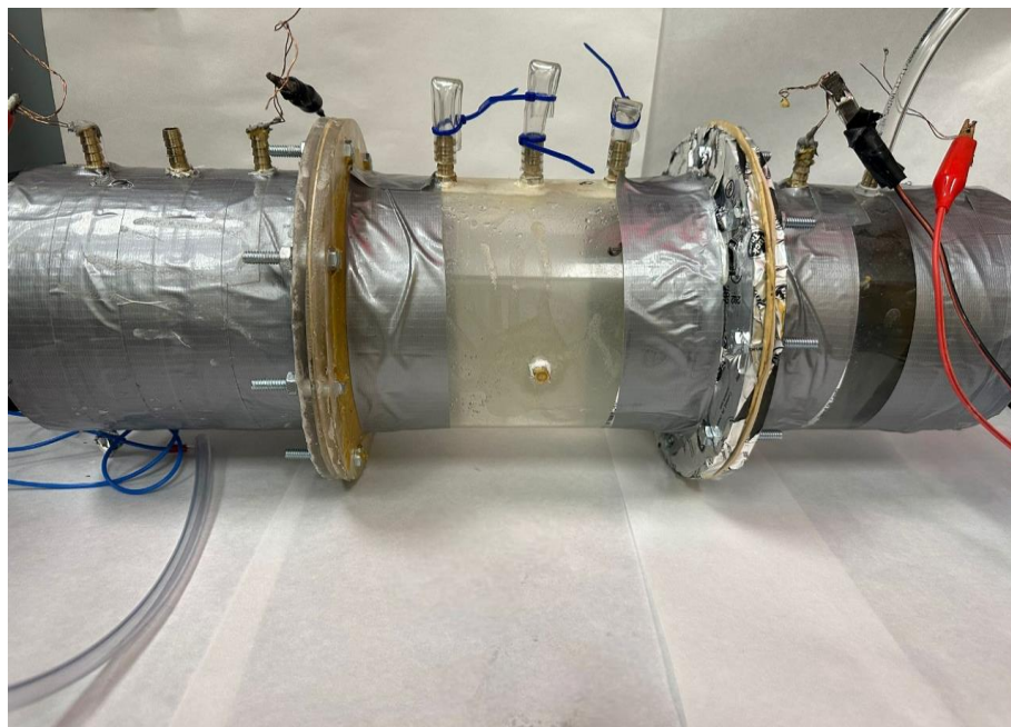
Figure 3.4 Front view of the designed reactor
