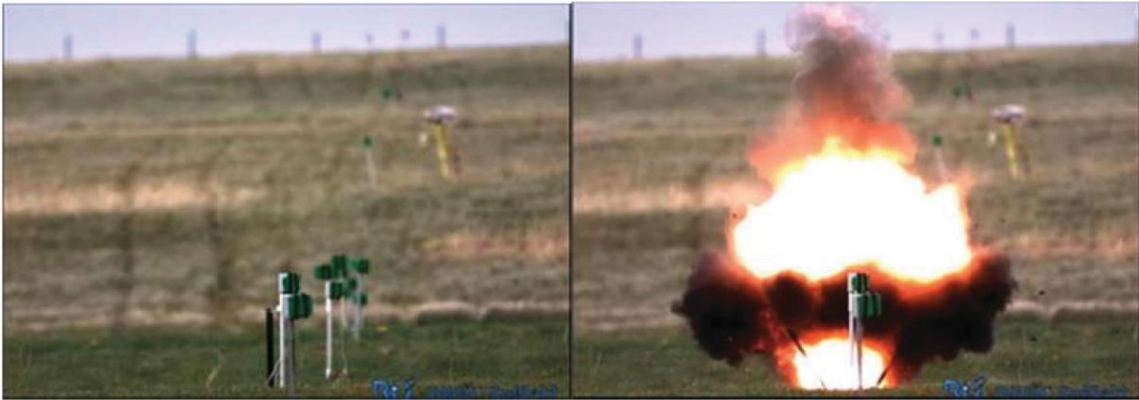
Figure 2: The photo on the left shows the GZ before the detonation, and the still photo taken from a high-speed camera on the right shows the fireball at its maximum size (Erhardt, Quayle, & Noel, Full-Scale RDD Experiments and Models, 2013).
