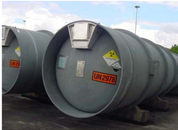
Figure 1.2: Photograph of a 48Y cylinder used to store \text{UF}_6 [14]. Dimensions of a 48Y cylinder are: 150" in length with a diameter of 48".
