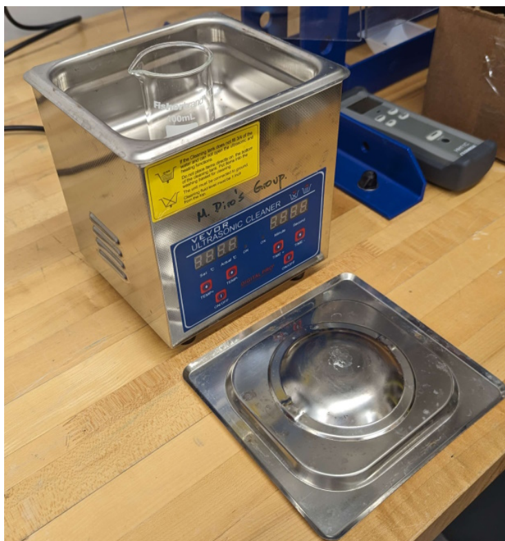
Figure 5.7: Photograph of Vevor Ultrasonic Cleaner used in this work for sample cleaning.
