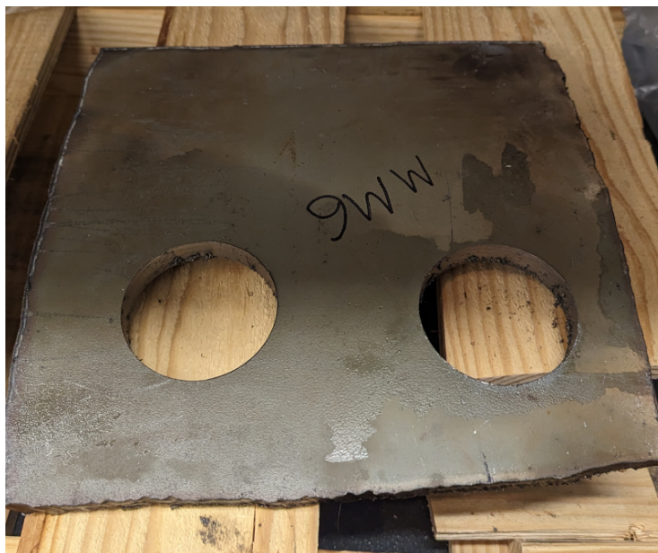
Figure 5.4: Photograph of full sample as received from Cameco Corporation with two cut out holes. Four plates were received, two large (18" x 18"), and two small (12" x 12").
