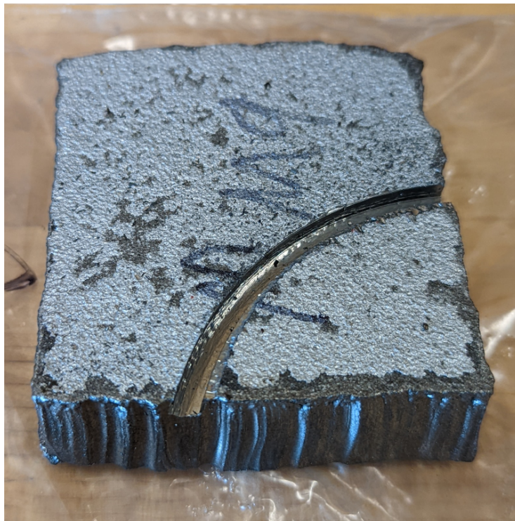
Figure 5.2: Photograph of small sand blasted sample after test cuts were made. The sample was difficult to cut through, and was stopped after it was decided high power equipment was required.
