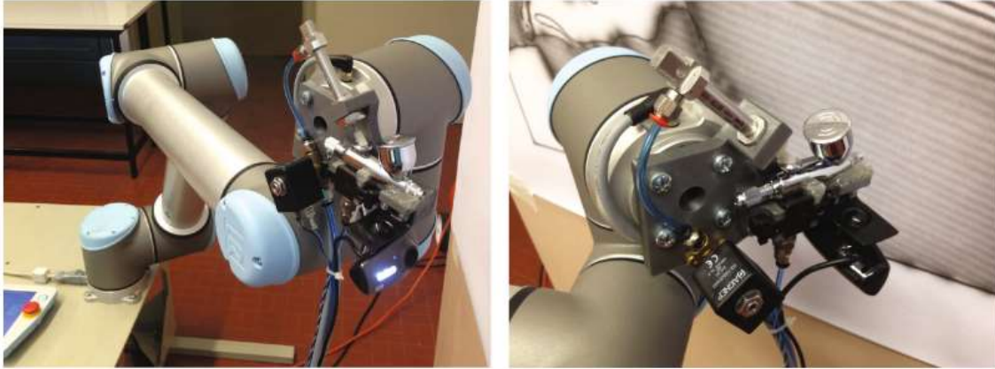
Figure 2.2: Integrated system for paint quality validation. [10]
