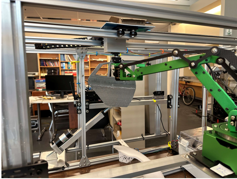
Figure 6.37: Robot executing trajectory on a car door.
