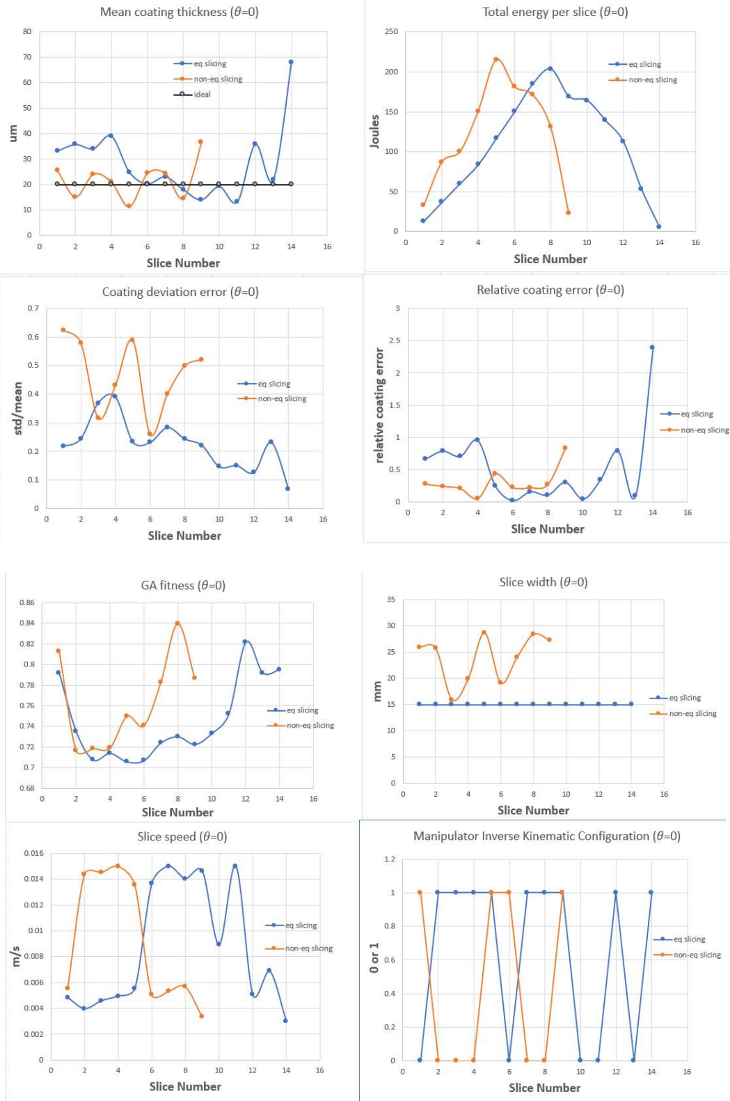
Figure 6.8: Mean coating thickness, energy, coating deviation and relative coating error, fitness, slice width, speed, and inverse kinematic configuration (car door: \theta = 0^\circ ).
