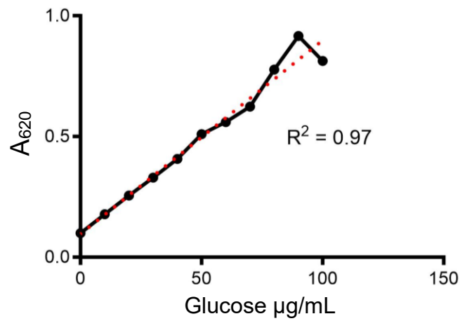
Figure A1. Standard curve for determination of glucose concentration in µg/mL). Experiments were done in triplicate n=3. R 2 value for line of best fit = 0.97.
