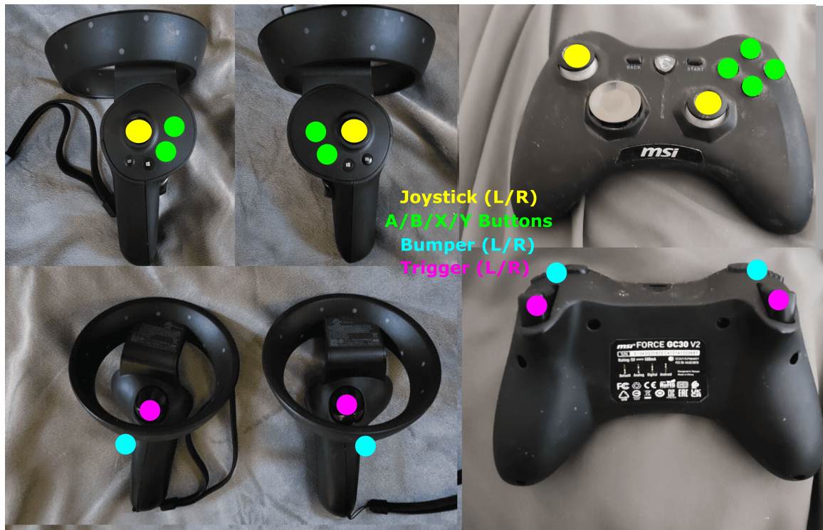
Figure 3: Gamepad and VR hand controller comparison, with labels
