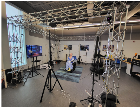
Figure 3.3: The Azure Kinects were mounted around the centre of the cube.
