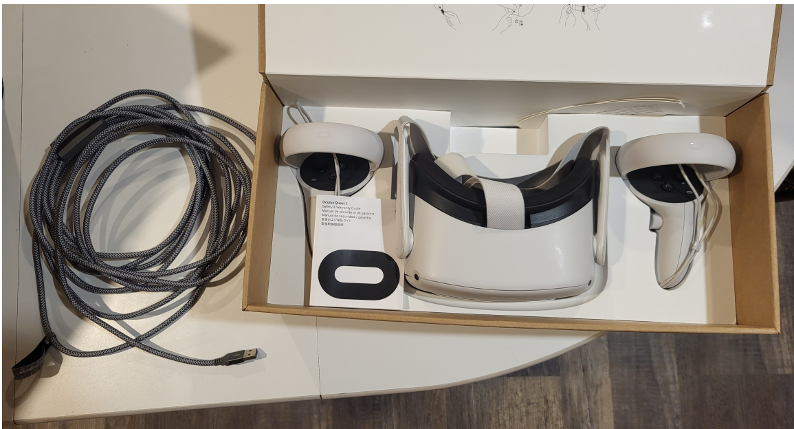
Figure 3.8: An Oculus Quest 2 was used for this study and an USB-C / USB-3 data link cable was used to connect the headset to the computer.
