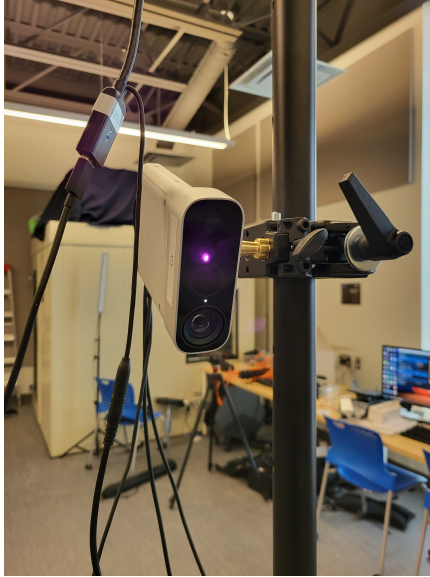
Figure 3.6: Mounting the camera horizontally may not be able to capture the full height of a person, therefore the camera is mounted vertically so that the wider field of view can be utilized more effectively.
