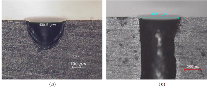
Figure 1.4: Difference in machining depth between (a) without using pulse voltage and vibrated electrolyte and (b) with pulse voltage and vibrated electrolyte. Republished with permission of Institute of Physics (IOP) Publishing, Ltd., from Geometric improvement of electrochemical discharge micro-drilling using an ultrasonic-vibrated electrolyte, Han et al., 19, 2009; permission conveyed through Copyright Clearance Center, Inc.
