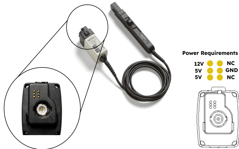
Figure 2.14: A layout describing the technical requirements for the current probe adapter. The current probe has 6 pads that need to be powered with specified signals, as indicated in the figure.
