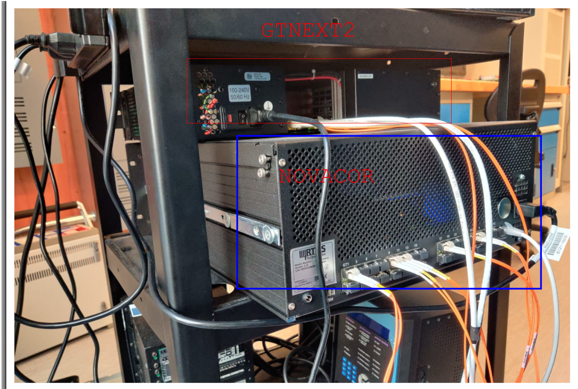
Figure 3.10: Hardware setup for modelling of centralized protection-Publisher
