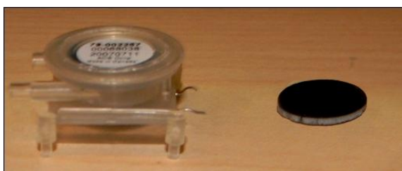
Figure 1.3: Commercially available breath alcohol sensor (on the left) and the fuel cell MEA that has been removed from a sensor cell (on the right)
