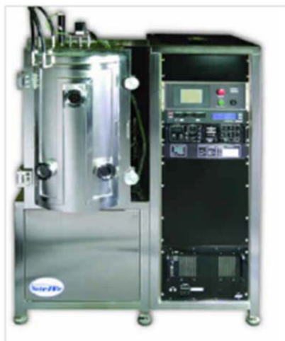
Figure 3.8: IntelVac Nanochrome I for electron beam deposition and DC sputtering
