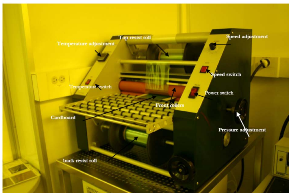
Figure 3.9: Bungard dry film laminator for sealing microchannels
