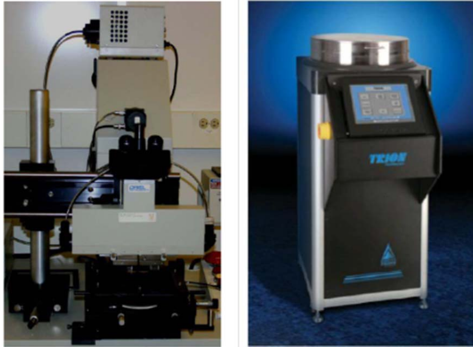
Figure 3.6: (a) UV mask aligner assembly for photolithography; (b) Trion Phantom II Plasma Etcher reactive ion etching
