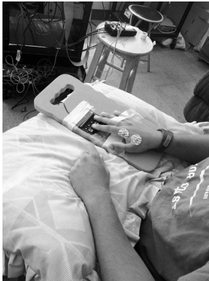
Figure 10. A custom keyboard was developed to allow the index finger to reach the 7, 8 and 9 keys of the numeric keypad. Other digits were then taped down in place to allow the proper hand orientation to allow the index finger to move freely and optimally activate the FDI muscle through abduction.
