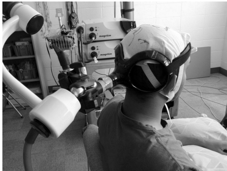
Figure 11. Cerebellar coil was positioned over the right hemisphere of the subjects cerebellum, and strapped in place around the subjects head to maintain a close fit.
